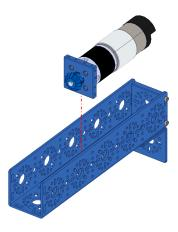
• Using 6 x M3 SHCS, screw the Orbital Motor Mount to the 240mm U-Channel.
